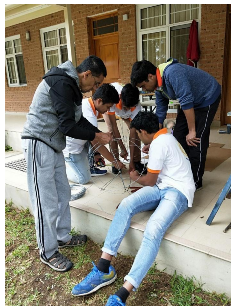
Winding the 5mm fibreglass rod helically around the body frame.
