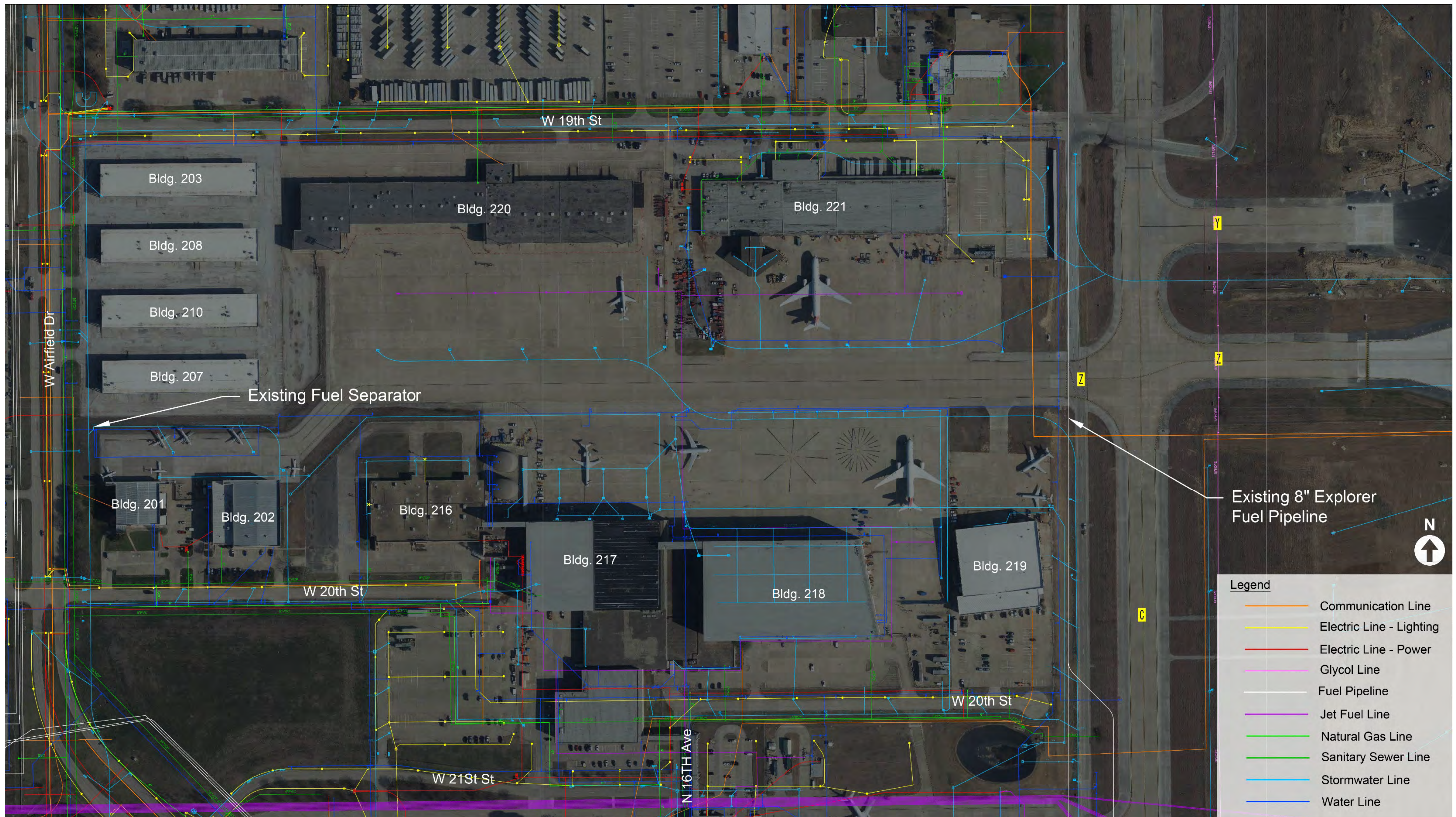
FIGURE 2-4 NW Cargo Campus Existing Utilities
