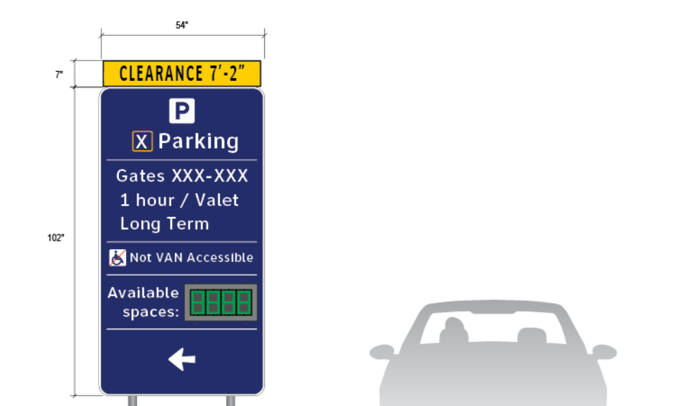
1 ELEVATION - Garage Entrance Area (Typical) Scale: 3/16" = 1'-0"
