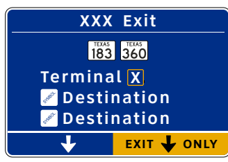
4-DR.12 Overhead 2-Lane 3-Line Directional Panel w/ Exit Header (27'-0" w x 18'-0" h)
