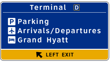
S-NB-2 Vehicular Directional Panel - Three Line Terminal (27'-0" w x 16'-6" h)
