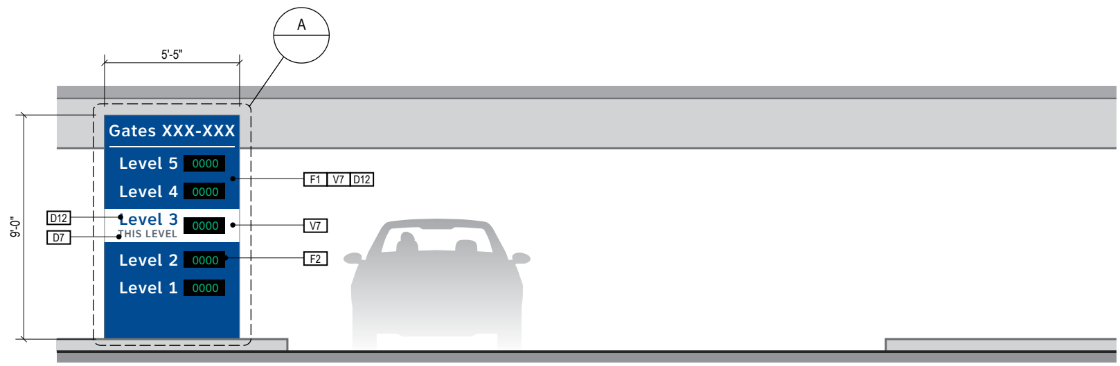
1 ELEVATION: Garage Level 3 Entrance Area (Typical) Scale: 3/16" = 1'-0"
