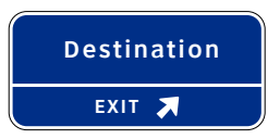
S-SB-10 Vehicular Directional Panel - Roadside (13'-0" w x 6'-0" h)
