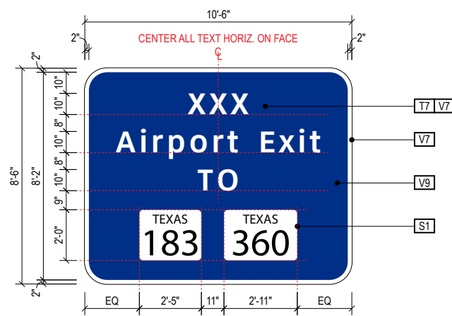
A7 FACE LAYOUT - *Typical Example (C-14-GM02 shown) Scale: 3/16" = 1'-0"
