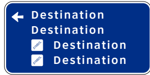
C-12-GM03 Vehicular Directional Panel - Roadside (16'-0" w x 8'-0" h)
