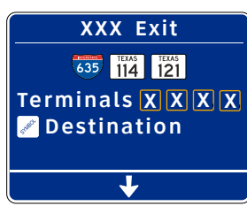
4-DR.11 Overhead 1-Lane 3-Line Directional Panel w/ Exit Header (23'-0" w x 18'-0" h)
