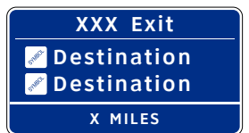
4-DR.06 Overhead Directional Mileage Panel w/ Exit Header (22'-0" w x 12'-0" h)
