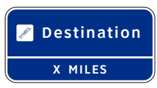
S-NB-11 Vehicular Directional Panel - Roadside (12'-0" w x 6'-0" h)
