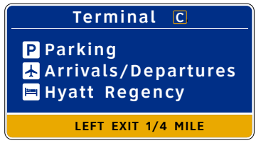
S-NB-2 Vehicular Directional Panel - Three Line Terminal (27'-0" w x 16'-6" h)
