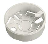
The Conduit Box is a versatile accessory for surface mounting Apollo bases. The box has knockouts to accept PG16 or M20 cable glands, conduit or mini-trunking. Self-tapping screws are included to fit the detector base to the conduit box.
