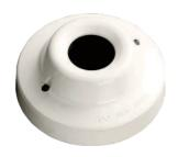
The Marine Intelligent Base Mounted IR³ Flame Detector is designed to protect all indoor areas, even in dirty or smoky conditions, where open flaming fires may be expected. The detector has three IR sensors that respond to different IR wavelengths to discriminate between flames and spurious sources of radiation.
