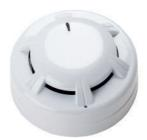
The Orbis Optical Smoke Detector operates on the well-established light scatter principle. The sensing technology used is radically different from previous optical detectors and significantly reduces false alarms.
