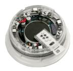
The XP95A Sounder Visual Indicator Base is a loop-powered sounder and visual indicator combined with a standard Intelligent Mounting Base. It is used to signal a fire alarm in enclosed areas. The sounder visual indicator base can be used either with a detector fitted or with a cap for operation as a stand-alone alarm device.
