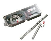
The Intelligent Duct Smoke Detector provides early detection of smoke in the air moving through heating and ventilation (HVAC) ducts in commercial and industrial premises. Its purpose is to prevent the re-circulation of smoke from an area on fire to areas unaffected by the fire when used with a XP95 or Discovery detector.
