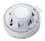
The XP95 I.S. Ionisation Smoke Detector uses a low activity radioactive foil to detect fires by irradiating the air in the smoke chamber and causing a current flow. If smoke enters the chamber, the current flow is reduced leading to an alarm.
