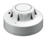
The Series 65 Ionisation Smoke Detector uses a low activity radioactive foil to detect fires by irradiating the air in the smoke chamber and causing a current flow. If smoke enters the chamber, the current flow is reduced leading to an alarm.
