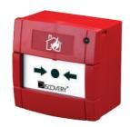
The Discovery Marine Manual Call Point has been approved for use in indoor marine applications. A seven-segment DIL switch enables addressing of each call point at commissioning stage. When operated, the manual call point interrupts the polling cycle for a fast response. Bi-coloured LEDs indicate isolate and normal conditions.
