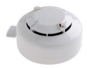
The Soteria Optical/Heat Multisensor Detector uses optical sensing technology, PureLight, to detect smoke particles entering the chamber and is fitted with two thermistors for detecting heat. It can be switched to detect smoke, heat or a combination of both, offering greater flexibility.
