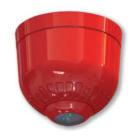
Conventional ceiling mounted Visual Alarm Devices are available with a white and red flash colour. The white flash variant has an EN 54-23 approved coverage pattern of C-3-15, whereas the red flash variant has a coverage pattern of C-3-8.9.
