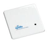
The XP95A 120V AC Input/Output module is a loop-powered device which incorporates a monitored input circuit for connection to dry contacts, in addition to a 120V AC 4A rated dry contact relay output. It is mounted in a plastic facia plate for use with a 42 square or two-gang electrical back box.
