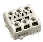
The Mini Monitor Module is an interface within an entirely new housing. This allows the unit to be fitted onto a standard 35mm DIN-Rail (using a twist-click motion) or mounted within an enclosure, for example a pull station. It is designed to monitor the state of one or more single pole, voltage-free contacts connected on a single pair of cables and to report this status to Apollocompatible analogue control equipment.
