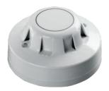
The AlarmSense Optical Smoke Detector works using the light scatter principle. The detector changes to alarm state at a pre-set threshold of smoke penetration into the sensing chamber.
