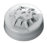
The Orbis Heat Detector monitors temperature by using a single thermistor which provides a voltage output proportional to the external air temperature.
