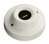
The Marine Intelligent Base Mounted UV IR² Flame Detector is designed to protect open indoor areas where open flaming fires may be expected. The detector has UV and dual IR sensors responding to different wavelengths to discriminate between flames and spurious sources of radiation.
