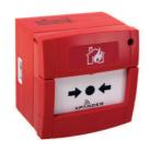
The XPander Manual Call Point is compliant with EN 54-11. It is wireless and is powered by two independent packs of three AA alkaline batteries with a typical five-year life.
