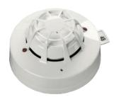
The XP95A Multisensor contains a photoelectric smoke sensor and a thermistor (temperature sensor) whose outputs are combined to give the final analogue value.
