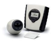
The high-performance Auto-Aligning Beam Detector comprises of a ground level controller, detector head with auto-aligning feature, integral laser for rapid initial alignment and single prism. An additional detector head can be added to the controller. Auto-Aligning Beam Detector is compatible with XP95 and Discovery, CoreProtocols®.
