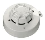
The Discovery UL Multisensor Detector consists of photoelectric smoke and thermistor temperature sensors whose outputs are combined to give the final analogue value. As a result, the multisensor is useful over a wide range of applications and is highly immune to false alarms.
