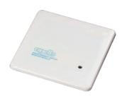
The XP95A Priority Switch Monitor Module is designed to monitor the state of one or more single pole, voltage-free contacts and to report this status to Apollo-compatible analogue control equipment. It can also place a signal on the loop to provide early warning if a device such as a pull station is operated.
