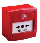
A seven-segment DIL switch enables addressing of each call point at commissioning stage. When operated, the manual call point interrupts the polling cycle for a fast response. Bi-coloured LEDs indicate isolate and normal conditions.
