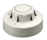
The Series 65A Photoelectric Smoke Detector incorporates a pulsing LED located within the housing of the detector. The detector has an indicator LED which is clear in a quiescent state but produces a red light when in alarm.
