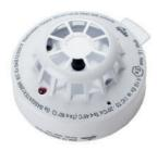
The XP95 I.S. Heat Detector operates by measuring heat levels with a single thermistor which gives an analogue value output proportional to the external air temperature.
