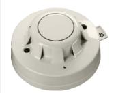
The Discovery UL Ionisation Detector uses a low activity radioactive foil to detect fires by irradiating the air in the smoke chambers and causing a current flow. If smoke enters the chamber, the current flow is reduced leading to an alarm.
