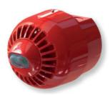
Conventional wall mounted Sounder Visual Alarm Devices are available with a white and red flash colour. The white flash variant has an EN 54-23 approved coverage pattern of W-3.1-11.3, whereas the red flash variant has a coverage pattern of W-2.4-7.5. The sounder has an a SPL of up to 97dB.
