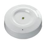
The Isolator is placed at intervals on the loop and ensures that, in the case of a short-circuit, only the section between the isolators will be affected. When the short-circuit is removed, the isolators automatically restore power and data to the isolated section.
