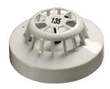
The Series 65A Heat Detector monitors temperature by using a dual thermistor network providing a voltage output proportional to the external air temperature. There are nine heat detectors in the Series 65A range designed to suit a wide variety of operating conditions.
