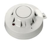
The XP95A Ionisation Smoke Detector uses a low activity radioactive foil to detect fires by irradiating the air in the smoke chambers causing a current flow. If smoke enters the chamber, the current flow is reduced leading to an alarm.
