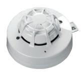
The Discovery Multisensor Detector comprises optical smoke and thermistor temperature sensors, which give both a combined signal as well as a separate heat signal for improved false alarm management.
