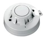
The Discovery Ionisation Smoke Detector uses a low activity radioactive foil to detect fires by irradiating the air in the smoke chambers and causing a current flow. If smoke enters the chamber, the current flow is reduced leading to an alarm.
