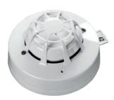
The Discovery Optical/Heat Multisensor Detector comprises optical smoke and thermistor temperature sensors which give both a combined signal as well as a separate heat signal for improved false alarm management.
