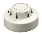
The Series 65A Ionisation Smoke Detector uses a low activity radioactive foil to detect fires by irradiating the air in the smoke chamber causing a current flow. If smoke enters the chamber, the current flow is reduced leading to an alarm.
