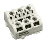
The Marine Mini Switch Monitor is an interface within an entirely new housing. Designed in response to customer feedback, the smaller Mini Switch Monitor can be fitted onto a 35mm DIN-Rail with a twist-click motion or mounted in an enclosure such as a manual call point. It is designed to monitor the state of one or more single pole, volt-free contacts connected to a single pair of cables and to report this status to Apollo-compatible control equipment.
