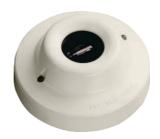
The Intelligent Base Mounted UV IR<sup>2</sup> Flame Detector is designed to protect open indoor areas such as aircraft hangers, generator rooms and paint works where open flaming fires may be expected. The detector has UV and dual IR sensors responding to different wavelengths in order to discriminate between flames and spurious sources of radiation.
