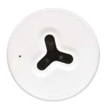
The innovative design of the Soteria Dimension Optical Detector differs from standard fire detectors, having no chamber and being flush mounted. A new optical sensing technology is used to detect smoke particles outside the detector housing. A combination of Infra-Red (IR) LEDs and photo-diodes identify smoke particles, detected just below the detector housing and initiates an alarm
