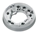
The TimeSaver® Relay Base incorporates a single-pole voltage-free changeover contact for switching external equipment. When the detector changes to the alarm state, the relay is energised, causing the contact to change state. The contact will remain in this condition until the detector is reset.
