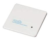
The XP95A Switch Monitor Input/Output Module provides a voltage-free, single pole, changeover relay output, a single, monitored switch input and unmonitored, non-polarised opto-coupled input.
