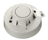
The Discovery Marine Ionisation Smoke Detector uses a low-activity radioactive foil to detect fires by irradiating the air in the smoke chamber and causing a current flow. If smoke enters the chamber, the current flow is reduced leading to an alarm.
