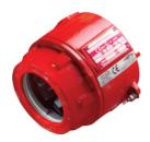
The Intelligent Flameproof IR³ Flame Detector is designed for hazardous environments in either indoor or outdoor applications. It is sensitive to low-frequency, flickering infra-red radiation emitted by flames during combustion. These detectors are BASEEFA approved and meet the requirements of ATEX Directive 94/9/EC.
