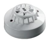
There are two heat detectors in the AlarmSense range designed to suit a wide variety of operating conditions. A static heat detector (CS) which responds only when a fixed temperature has been reached and a rate-of-rise detector (A1R) which has a fixed upper limit, but in addition, measures the rate of increase in temperature.
