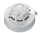
The XP95 Optical/Heat Multisensor Detector contains an optical smoke sensor and a thermistor temperature sensor whose outputs are combined to give the final analogue value.
