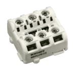
The Mini Switch Monitor is an interface within an entirely new housing. This allows the unit to be fitted onto a standard 35mm DIN-Rail (using a twist-click motion) or mounted within an enclosure for example, a manual call point. It is designed to monitor the state of one or more single pole, volt-free contacts connected on a single pair of cables and to report this status to Apollo-compatible analogue addressable control equipment.
