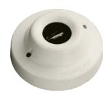
The Marine Intelligent Base Mounted UV Flame Detector is designed to protect enclosed indoor areas where open fires may be expected. The detector has a fast-acting response to flames up to 25m away and is equipped with a single UV sensor with a narrow spectral response to discriminate between flames and most spurious sources of radiation.
