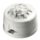
There are two heat detectors in the XPander range, designed to suit a wide variety of operating conditions. A Static Heat Detector (CS) which responds only when a fixed temperature has been reached and a Rate-of-Rise Detector (A1R) which has a fixed upper limit, but in addition, measures the rate of increase in temperature.
