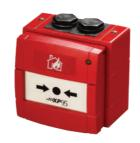
The Waterproof Manual Call Point has been designed for use outdoors and in places where moisture can occur. A seven-segment DIL switch enables addressing of each call point at commissioning stage. When operated, the manual call point interrupts the polling cycle for a fast response. Bi-coloured LEDs indicate isolate and normal conditions.
