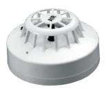
The Series 65 Heat Detector monitors temperature by using a dual thermistor network which provides a voltage output proportional to the external air temperature.
