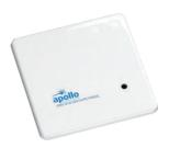
The XP95A 120V AC Input/Output module is a loop-powered device which incorporates a monitored input circuit for connection to dry contacts, as well as a 120V AC 4A rated dry contact relay output. It is mounted in a plastic facia plate for use with a 42 square or two-gang electrical back box.
