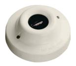
The Intelligent Base Mounted UV Flame Detector is designed to protect enclosed indoor areas where open fires may be expected. The detector has a fast-acting response to flames up to 25m away and is equipped with a single UV sensor with a narrow spectral response in order to discriminate between flames and most spurious sources of radiation.
