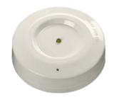
The Discovery Marine Isolator is placed at intervals on the loop and ensures that, in the case of a short-circuit, only the section between the isolators will be affected. When the short-circuit is removed, the isolators automatically restore power and data to the isolated section.
