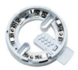
All detectors in the Soteria, Discovery and XP95 ranges fit into the XPERT 8 Intelligent Mounting Base. The base has a wide interior diameter for ease of access to cables and terminals. Additionally, the detector can be locked into the base for increased security, with a grub screw using a 1.5mm hexagonal driver. The XPERT 8 card, part number 38532-064, supplied with the base, has pre-punched pips to remove to set the address.
