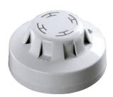
Ionisation detectors use a low activity radioactive foil to detect fires by irradiating the air in the smoke chamber and causing a current flow. If smoke enters the chamber, the current flow is reduced leading to an alarm. Circuitry in the Integrating Ionisation Smoke Detector protects against transient levels of smoke above the normal threshold for up to 20 seconds.
