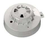
The XP95A Heat Detector monitors temperature by using a single thermistor which provides a voltage output proportional to the external air temperature. It is classified as an ordinary detector by UL.
