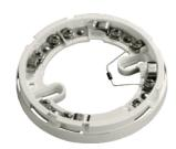
The Series 65 Diode Base is designed for use with conventional systems that have manual call points and detector bases on the same circuit. The base is fitted with a schottky diode on the 'L1 IN' and 'L1 OUT' wiring terminals. This base can only be used with compatible control equipment.
