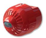
Conventional wall mounted Visual Alarm Devices are available with a white and red flash colour. The white flash variant has an EN 54-23 approved coverage pattern of W-3.1-11.3, whereas the red flash variant has a coverage pattern of W-2.4-7.5.
