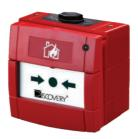
The Discovery Marine Manual Call Point has been approved for use in outdoor marine applications. A seven-segment DIL switch enables addressing of each call point at commissioning stage. When operated, the manual call point interrupts the polling cycle for a fast response. Bi-coloured LEDs indicate isolate and normal conditions.
