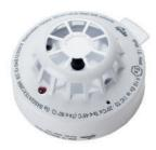
The XP95 I.S. Heat Detector operates by measuring heat levels with a single thermistor which gives a count output proportional to the external air temperature.
