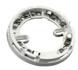
The Series 65 Standard Base has been designed to enable detectors to be fitted without the need of force – particularly useful when fitting to suspended ceilings. All Series 65 bases have a one-way only fit. Detectors can be locked into place by a grub screw using a 1.5mm hexagonal screwdriver.
