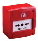
The Discovery Manual Call Point has a seven-segment DIL switch enables addressing of each call point at commissioning stage. When operated, the manual call point interrupts the polling cycle for a fast response. Bi-coloured LEDs indicate isolate and normal conditions.
