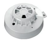
The Discovery Heat Detector uses a single thermistor to sense the air temperature around the detector.
