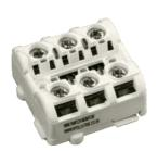
The Marine Mini Switch Monitor is an interface within an entirely new housing. Designed in response to customer feedback, the smaller Mini Switch Monitor can be fitted onto a 35mm DIN-Rail with a twist-click motion or mounted in an enclosure such as a manual call point. It is designed to monitor the state of one or more single pole, volt-free contacts connected to a single pair of cables and to report the status to Apollo-compatible control equipment.
