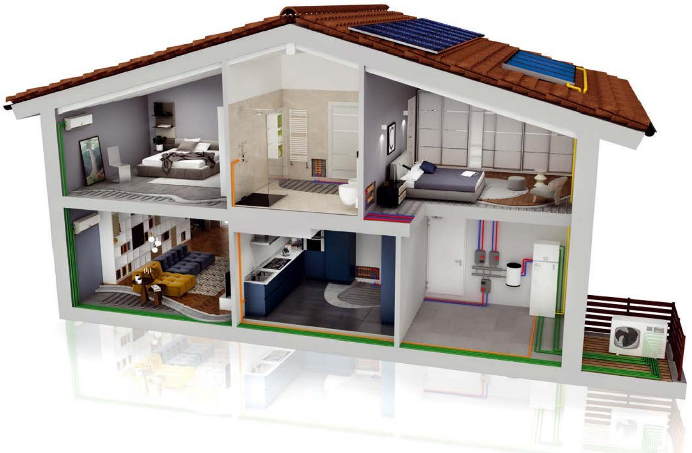
„AQUA UNIT“ – NAUJOJI „ISERIES“ SISTEMOS PATALPŲ VIDUJE MONTUOJAMA VANDENINĖ DALIS, SKIRTA ŠILDYMO IR VĖSINIMO SPRENDIMAMS ĮGYVENDINTI PATALPOSE SU GRINDŲ ŠILDYMO SISTEMA, SIENINIAIS, LUBINIAIS IR PASTATOMAIS RADIATORIAIS AR VENTILIATORINIAIS KONVEKTORIAIS.
