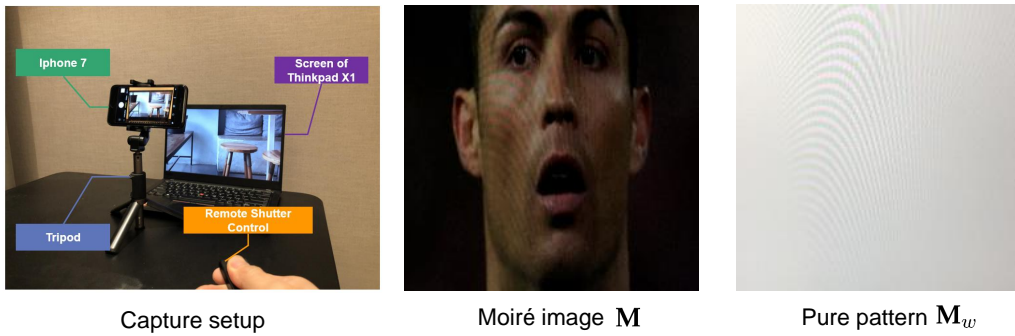
Figure 2: The data capture setup for moiré pattern extraction (Left), and an additional example of captured image pairs (Middle and Right).
