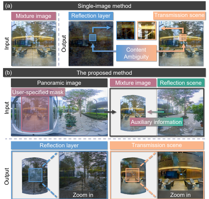
Fig. 1: Illustration of different setups of the single-image reflection removal method (we show the result from [4] as an example) and the proposed method. (a) The single-image method only inputs with a mixture image, and fails in distinguishing the reflection layer and transmission scene due to the content ambiguity. (b) The proposed method inputs with a panoramic image and a user-specified mask, which utilizes auxiliary reflection content information to relieve the content ambiguity, and recovers the much clearer reflection layer and transmission scene than (a).
