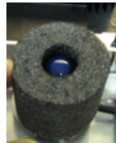
Photo Cell for Auto Dimming with Protective Shielding
