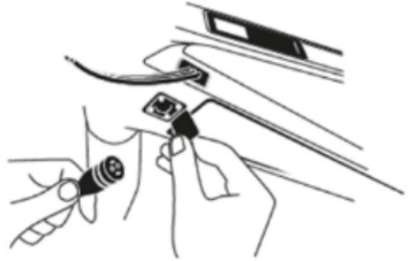
**Charging the battery inside the S-Pedalec:**
