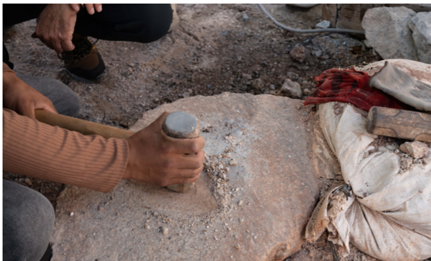
Gualberto Urbina, Legal Representative of Minera Estrella del Sur and Zosani Cruz, in Minera Virgen del Chapi, crushing gold-bearing ore captured during the field mission in Peru
