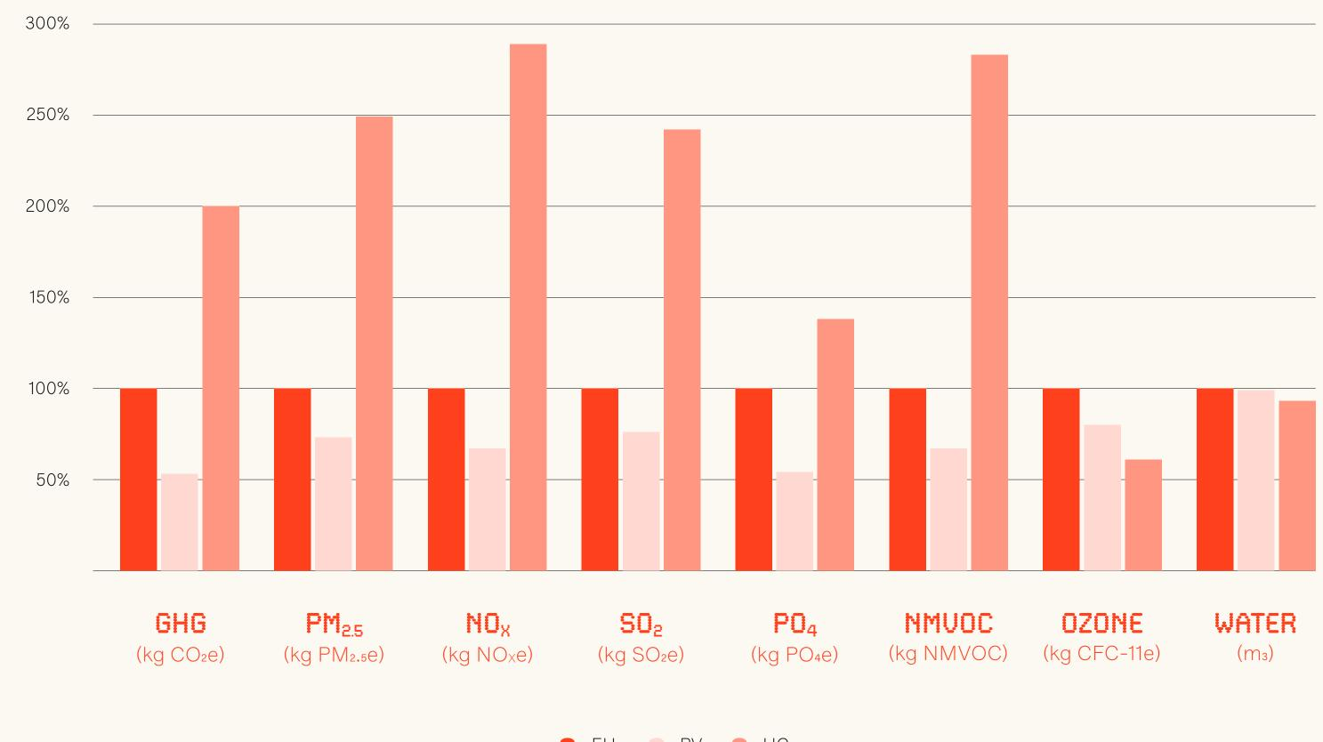
Environmental impact of Instagrid ONE considering different sources of energy, for example the EU standard electricity mix vs PV solar energy vs coal-based energy.
