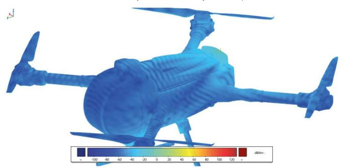
Figure 3: Induced Currents on a Colibri Drone
