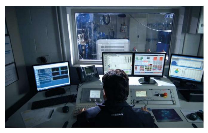
accelerates testing by realistically simulating the damage experienced by the component during the operational life of the vehicle.
