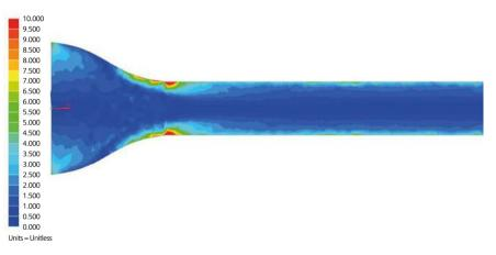
Figure 6: CFD simulation using Simcenter 3D Flow and Simcenter 3D Thermal was used to optimize the geometry of the wind tunnel asa hydraulik built at its headquarters in Vienna, Austria
