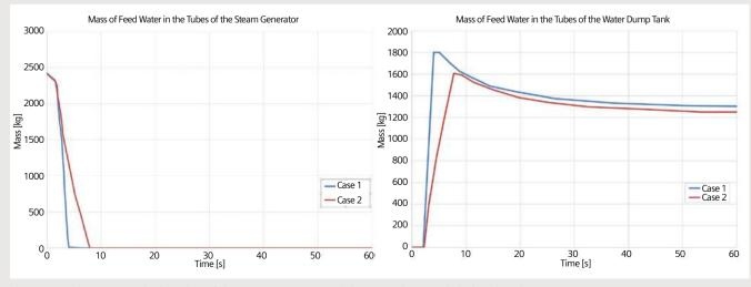
Figure 3. Feed water mass in the tubes of the steam generator and the water dump tank during shut-down
