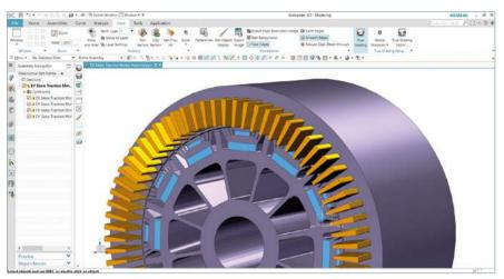
Figure 2: Skewed EV Traction Motor assembly in Simcenter 3D
