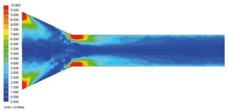
Kontraktion\_stp\_fem1\_sim1: Solution 2 Result Load Case 1, Static Step 1 Vorticity - Element-Nodal, Unaveraged, Magnitude Min: 0.04, Max: 34.20, Units = Unitless
