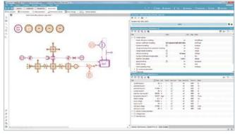
Figure 2: Simcenter Amesim battery model
