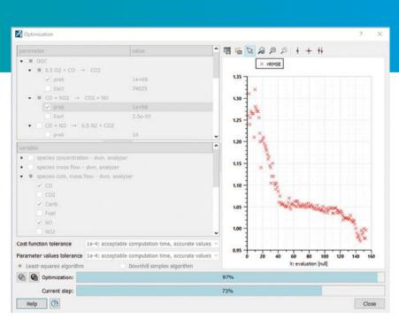
Figure 2: The optimization feature helps the kinetic model calibration
