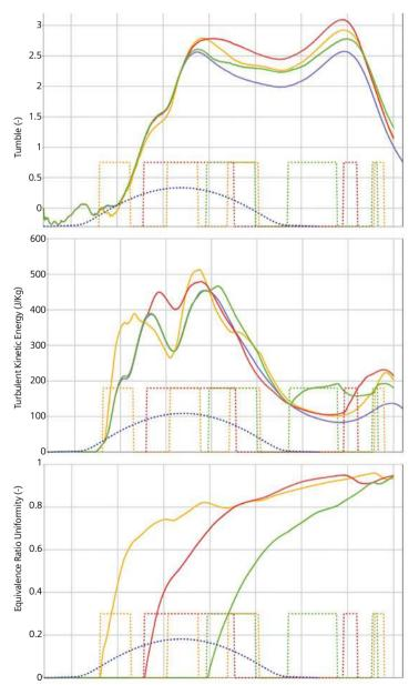
Figure 2: Transient evolution of averaged tumble, turbulence and equivalence ratio uniformity for three selected candidate injection strategies (dotted lines)
