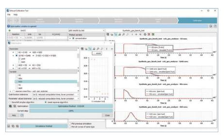
Figure 1: Simcenter Amesim Exhaust calibration tool is an interactive interface with a step by step workflow
