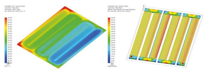
Figure 5: asa hydraulik uses Simcenter 3D Flow and Simcenter 3D Thermal from Siemens Digital Industries Software for computational fluid dynamics (CFD) simulations, optimizing their designs for temperature progression (left) and flow velocity (right), among other criteria
