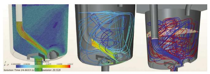
Figure 6: Simcenter STAR-CCM+ simulations showing velocity vectors, flow streamlines and particle tracks in the sump, indicating little short-circuiting and quick dissipation of the recirculating flow by the impeller
