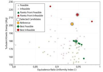
Figure 1: Trade-off between turbulent kinetic energy and fuel distribution homogeneity at ignition timing for 80 different multi-pulse injection strategies
