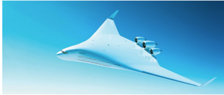
Figure 2. The increased fuselage space of blended wing body aircraft can be used to store batteries, hydrogen or hydrogen and fuel cells without sacrificing passenger or cargo capacity.
