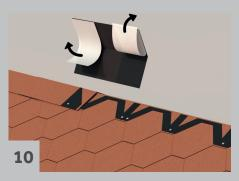
The top row of shingles should be positioned sufficiently far up against the ridge that the ridge plates can reach down to the bottom of the incision. The perforations divide the eave/ridge plate into three ridge plates.
