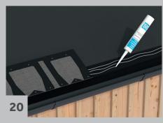
The eave plate should be laid parallel along the eaves. String should be used to maintain the alignment. 3 lines of Icopal Roof Glue should be applied to the fitting.
