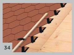
The easiest way to laterally insert new shingle is through marking out a join.
