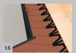
On roofs with protrusions, the part of the roof protruding furthest will determine both "up/down" and sideways directions. Start laying as shown in figures 1-3. Lay the shingle up to the next eaves and fit base plates as shown in fig. 1. Shift the base plates to the side so that the adhesive fields fit in relation to the shingle tongues. Continue to maintain the height and direction of the shingle sheets. Shingles protruding from the underside of the eave plates should be cut.
