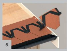
At the rake, the shingles should be bent up onto the batten and stapled. The nails will be covered by the next shingle sheet. Then cut the shingle along the rake.
