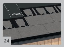
The next row is added to the second so that the lower edge of the tongues is flush with the bottom of the incision in the previous row. Continue laying upwards.
