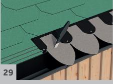
Lay a shingle sheet facing upward on the bottom of the second row of the old roofing. Secure with three lines of Icopal Roof Glue and cut at the eaves. Staple down the upper securing strip.
