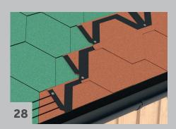
Continue laying in the same way as with shingles on a new roof. See point 4 and the following points. If individual tongues from the old roofing are protruding too far down, cut the excess cut off.
