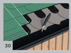
Mark two parallel lines with chalk approximately in the middle of the roof. The distance should be equal to the width of half of the tongue of the shingle. Lay the next row on the bottom of row three in the old roofing. Tack in the adhesive field and cut at the eaves. Further laying is guided throughout by the lower edge of the tongues on the old roofing.
