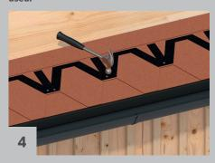
The shingle should be stapled to the substrate approx. 2.5 cm above each incision. It should be stapled to the adhesive field on each side of the joint. Then lay each row so that the lower edge of the tongues aligns with the bottom of the incisions in the previous row.
