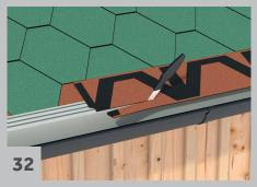
Start as shown in figure 25. Fit the new covering. Apply three lines of glue to the covering. The lateral joint should be in the middle of the underlying tongue and make sure that the new shingle is always on the underside of the tongues on the next row of old shingles. The sheet is attached with one pin on each securing strip and two nails at the joint. Cut at the eave plate.
