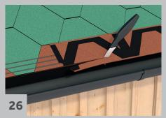
Lay the rest of the shingle sheet the right way onto the row of old shingle. The lateral joint should be in the middle of the underlying tongue. Attach the new sheet with a nail in each securing strip. Lay three strips of Icopal Roof Glue and cut at the eaves.
