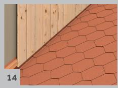
When joining up to a wall, a triangular batten should be used. Up to 15 cm of the covering should be laid on the wall. The top edge should be covered with cladding or fittings.
