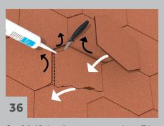
Carefully lift the adjacent tongues and cut off the damaged part, 15-20 mm inside the edge. Make an identical piece and put it in place. Use plenty of Icopal Roof Glue and tread into place. The plate should not be nailed.
