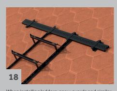
When installing ladders, snow guards and similar to the roof, it is important to seal the screws under the mounting bracket with Icopal Roof Glue to prevent leakage. All attachment points on the shingles should be centred as much as possible.
