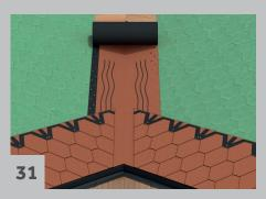
Cut off old shingling and coatings from the valley approx. 50 cm from the centre of the valley. In the valley, lay a roll of roof membrane of the same colour of a width of 1 metre. The roll should be stapled on both sides, with approx. 6 cm between the nails. Mark the valley width, approx. 15 cm on each side and apply three lines of Icopal Roof Glue. Also see fig. 17.
