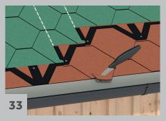
Mark two parallel lines with chalk approximately in the middle of the roof. The distance should be equal to the width of half of the tongue of the shingle. Lay the next row of shingle sheeting onto the next row of old shingle. Attach the new sheet with a nail in each securing strip. Cut at the eave plate. Continue laying in the same way so that the new shingle is constantly on the underside of the tongues in the next row of old shingles. Follow the existing pattern.
