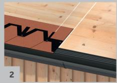
Mark two parallel lines with chalk approximately in the middle of the roof. The distance should be equal to the width of half of the tongue of the shingle. Start laying one row of the shingles and continue towards the sides. The next row should start by the other row.
