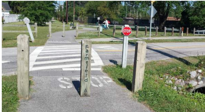
Closely-spaced bollards at street crossings on the Greenway create hazards for bicyclists.
