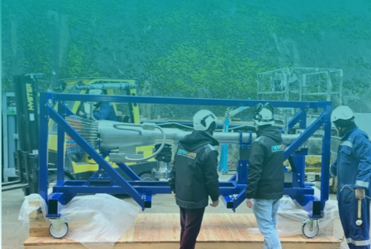
2MW core simulator part of OTHELLO facility
