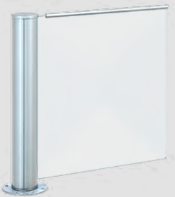
Charon HSD-E03 Half-height swing door with glass element, TSG, 10 mm top edge, 900 mm door leaf
