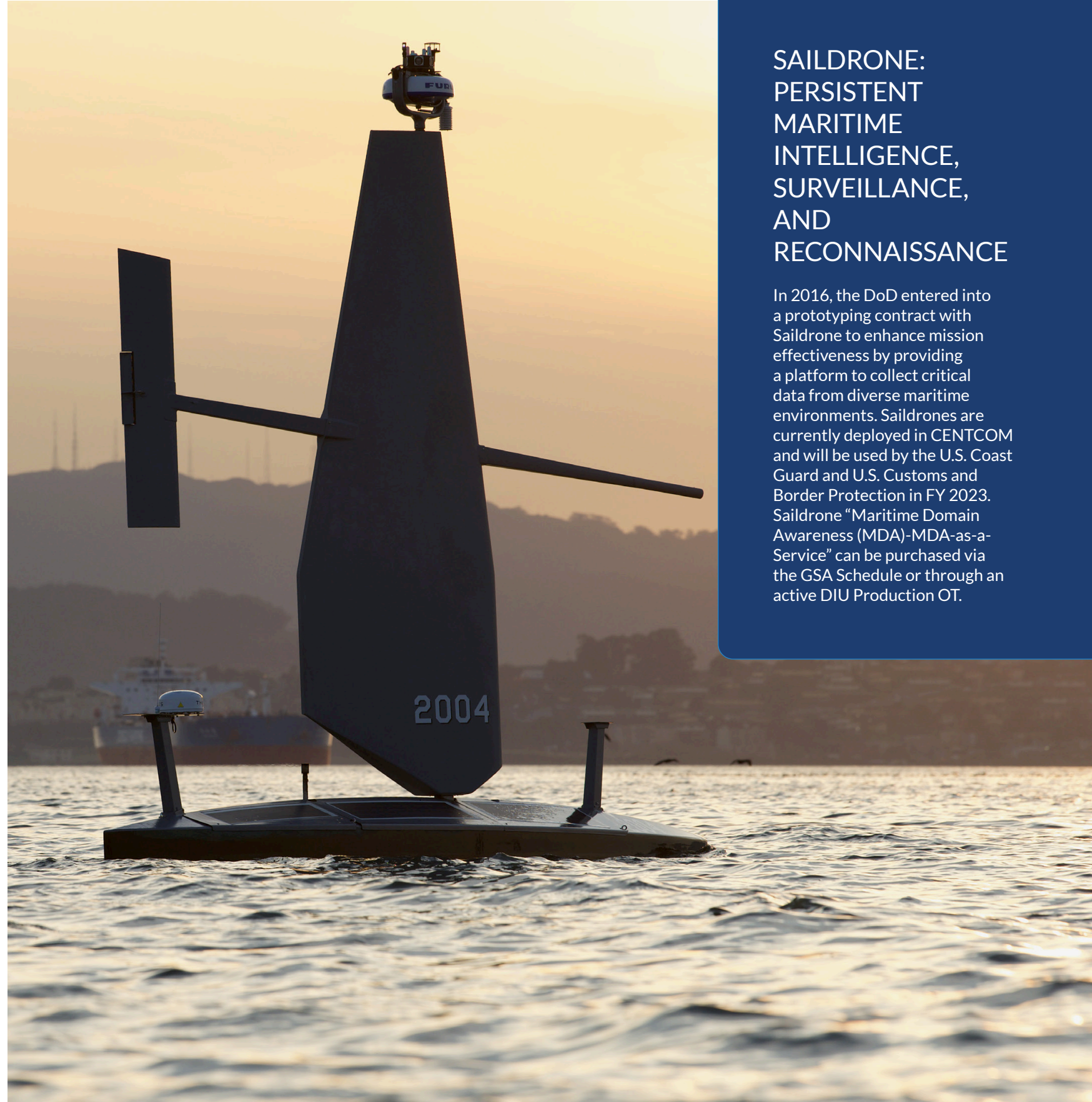
Saildrone "Voyager" model undergoing sea trials in the San Francisco Bay. Voyagers are specifically designed for ultra long endurance Maritime Domain Awareness (MDA) (Source: Saildrone)
