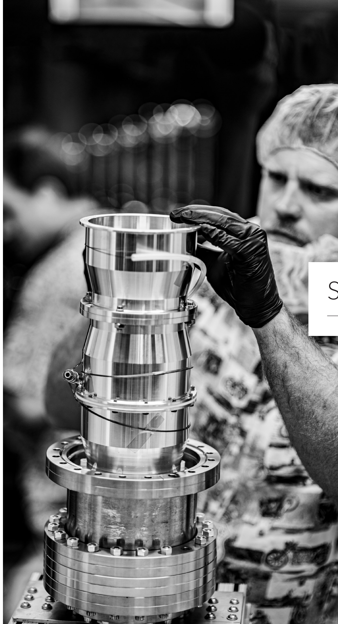
An Avalanche Energy scientist works to assemble the fusion reactor core 'Neo', the first of several planned iterations that utilizes a unique electrostatic plasma confinement technique called an 'Orbitron' (Source: Avalanche Energy Designs)
