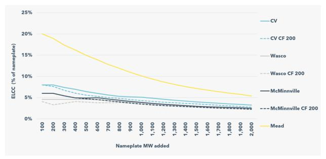
**Figure 147** and **Figure 148** shows storage ELCC values.<sup>491</sup> Note that with pumped storage hydropower, the model entirely solves all adequacy issues before reaching the 2,000 MW
