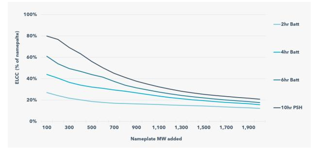
**Figure 149** and **Figure 150** shows hybrid resource ELCC values. Some hybrid resources solve all adequacy issues before reaching the 2,000 MW nameplate of the resource. Once the model solves out, ELCC values are reduced by 1 percent for each subsequent 100 MW of resource.
