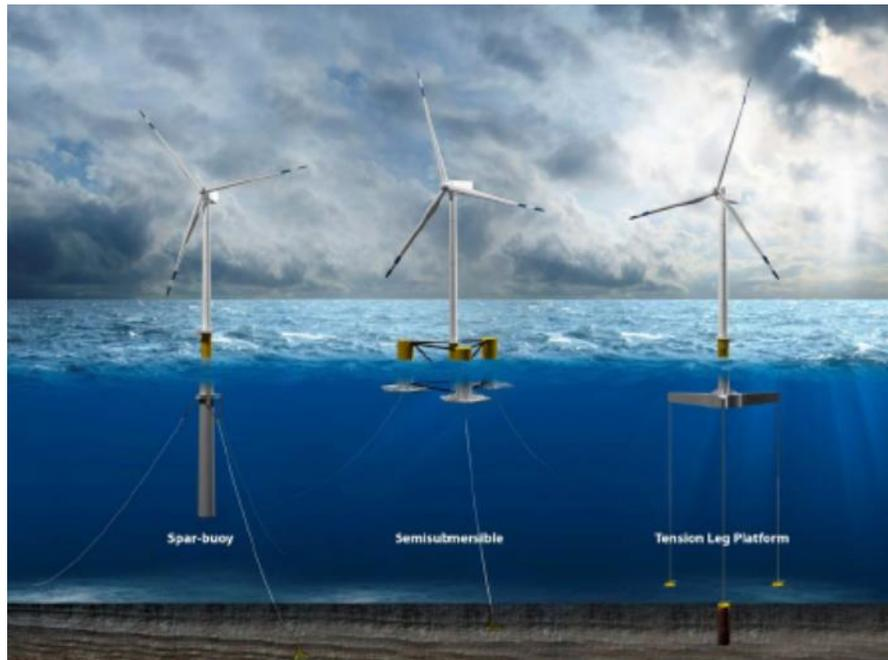
The assumption for a project online in 2032 makes use of semi-submersible platforms employing turbines rated at 15 MW with 248-meter rotor diameters at hub heights of 150 meters. These specifications are equivalent to those proposed by NREL for the 2032 reference technology. Turbine power curve data are also consistent with those used by NREL, as updated for 2021.<sup>506</sup>
