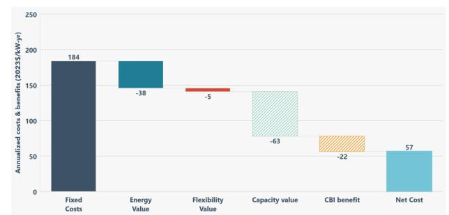
Figure 77. Net cost of a microgrid CBRE (2026 COD)
