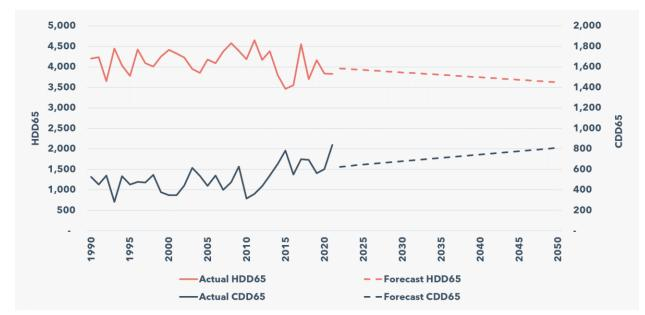
Figure 115. Normal weather expectation in terms of heating degree days and cooling degree days
