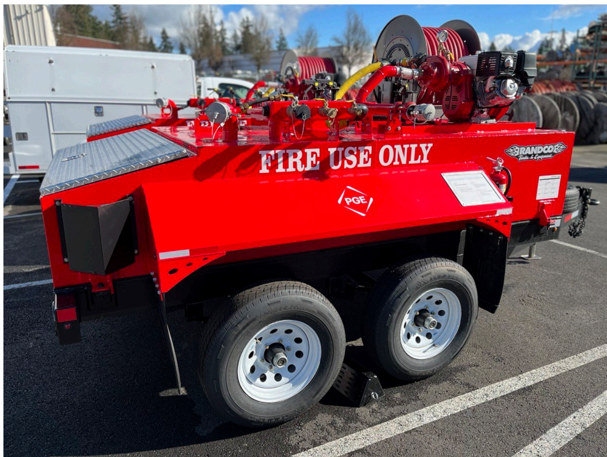
Figure 10-1: 500 Gallon Mobile Fire Trailer
