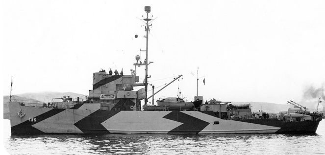
USS Admirable (AM-136) the lead ship of her class. Note: WWI style dazzle paint camouflage pattern.
