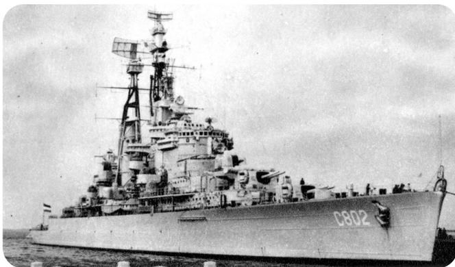
In August 1976 *De Zeven Provinciën* was renamed *Aguirre*. RIM-2 Terrier SAM removed, replaced by a hangar with large flight deck for three ASH-3D Sea King helicopters. Decommissioned 1999.
