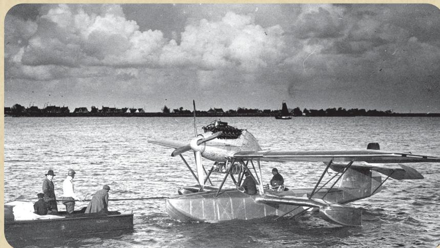
*A significantly more ambitious project was the B.II amphibian. It featured a metal flying boat hull housing a crew of three. The sesquiplane was powered by a 360 HP Rolls Royce Eagle IX engine. It was designed to be used from projected navy cruisers. After completing its test flights, it was offered to the navy for trials, but it did not meet expectations and was rejected.*
