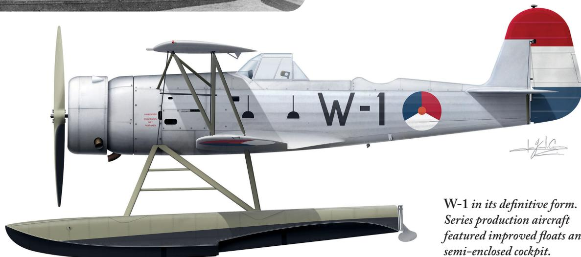
*W-1 in its definitive form. Series production aircraft featured improved floats and a semi-enclosed cockpit.*
