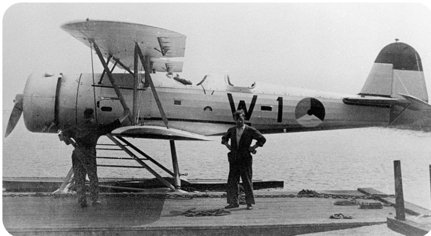
*The prototype before a flight to Germany. Its civil registry is not yet applied, but the gun ring is removed, and the rear cockpit coaming is modified. (Collection: N. Braas)*
