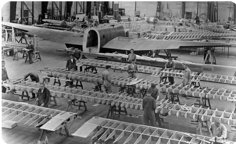
*In the front of the picture a pair of lower wings can be seen, with three top wings behind. In the background, Fokker T.V wings are being built, which also included the fuselage centre section.*
