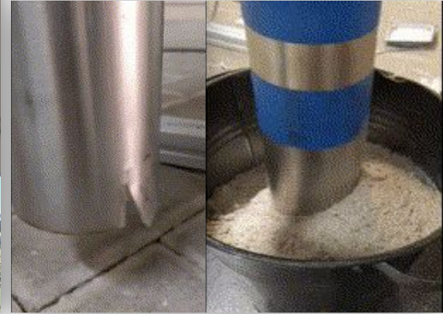
Bottom section rotating without (left) and with (right) sand and screw
