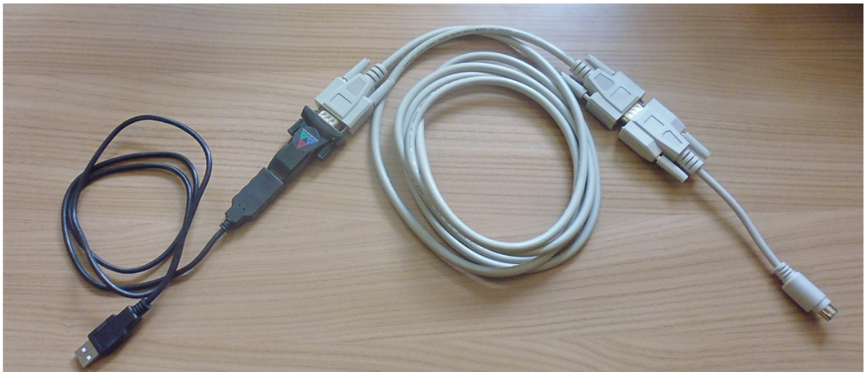
8 : RS-232 connection arrangement using USB and mini-DIN adaptors.
