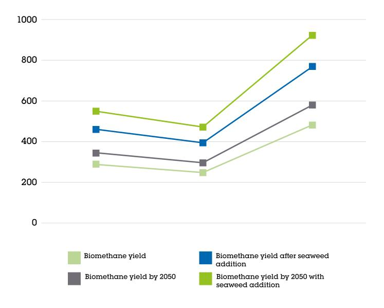
**Figure 3.** Green Gas potential of the UK (TWh). It is assumed that the addition of seaweed increases methane yield by 20%. Figure 3 represents that grey line is 20% higher than pale green line; and bright green line is 20% greater than blue line.
