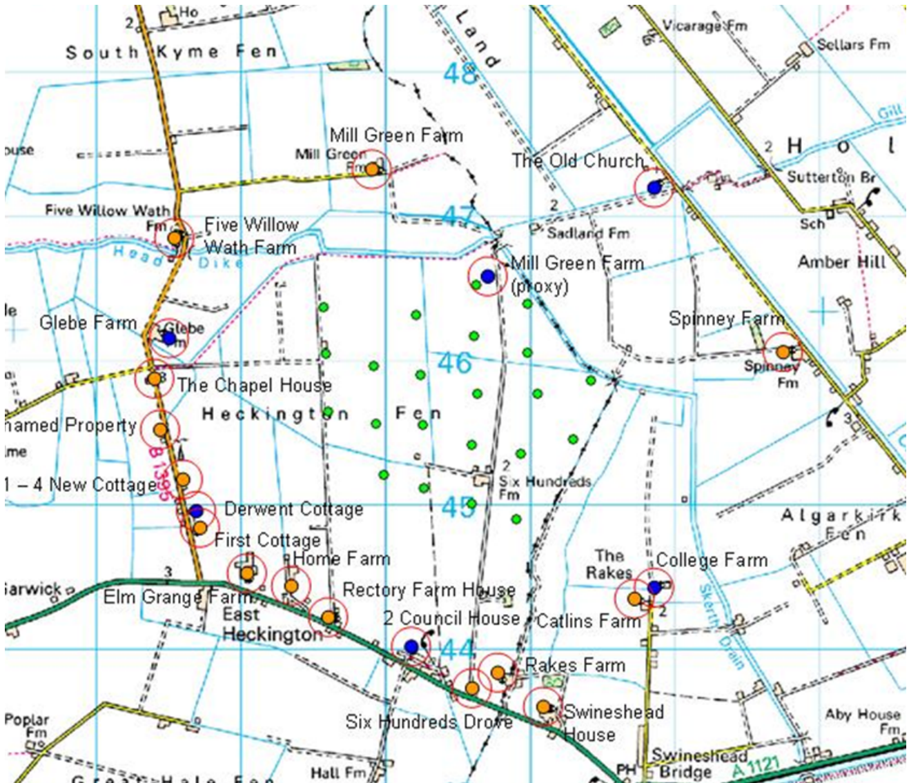
Figure 12.1.2 – Historical March 2011 Background noise survey locations (blue) and noise sensitive receptor locations (orange) from the Heckington Fen Wind Park application.
