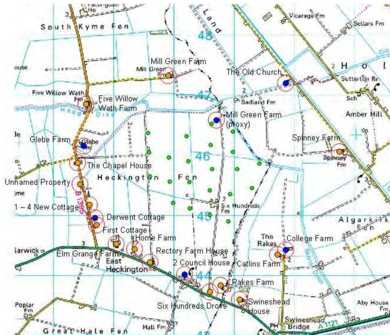
Figure B1 Map showing the layout of the turbines (green dots), the noise monitoring locations (blue dots within red circles), the additional noise assessment locations (orange dots within red circles).
