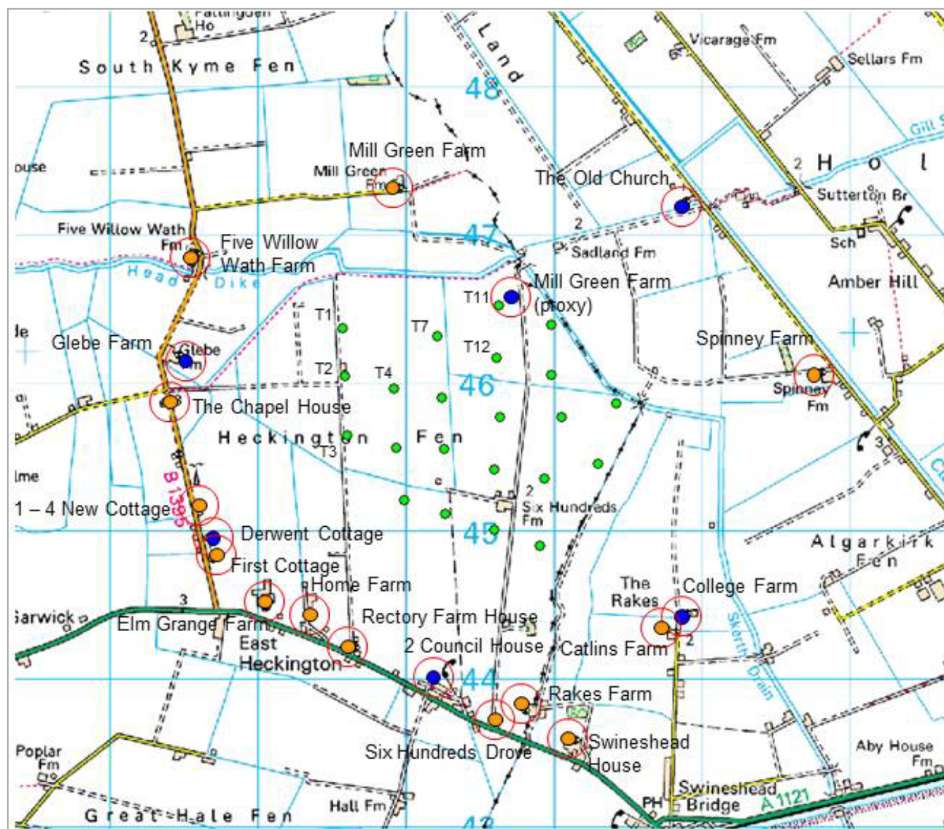
Figure A1: Map showing the layout of the Siemens SWT-101 turbines (green dots), the noise monitoring locations (blue dots within red circles) and the additional noise assessment locations (orange dots within red circles).
