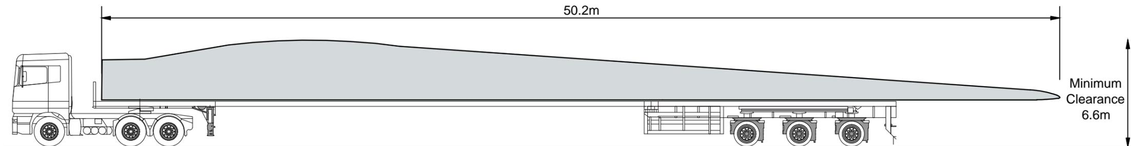
Final transport vehicle configuration to depend on turbine supplier and transport company requirements
