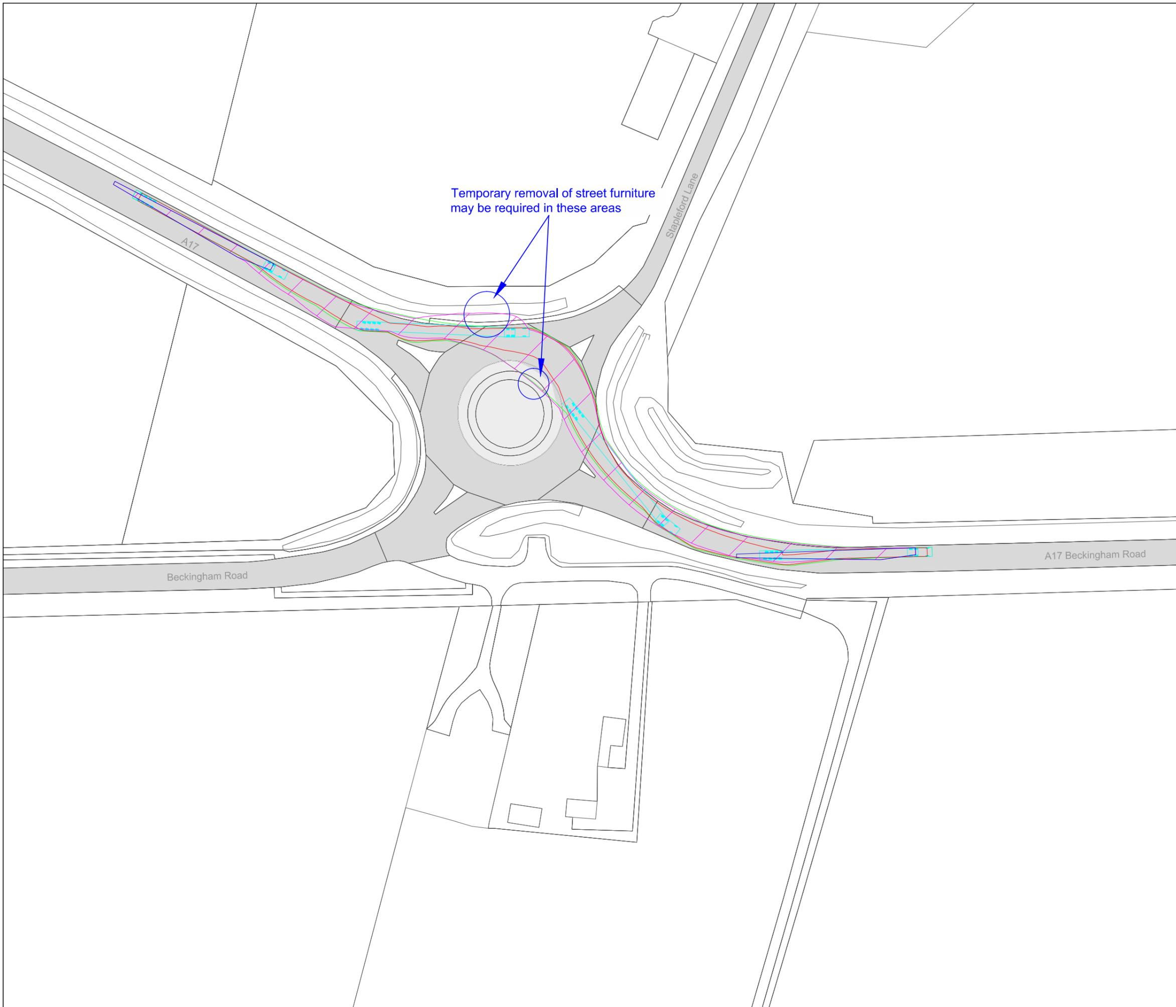
Swept path undertaken using rear axle steering
