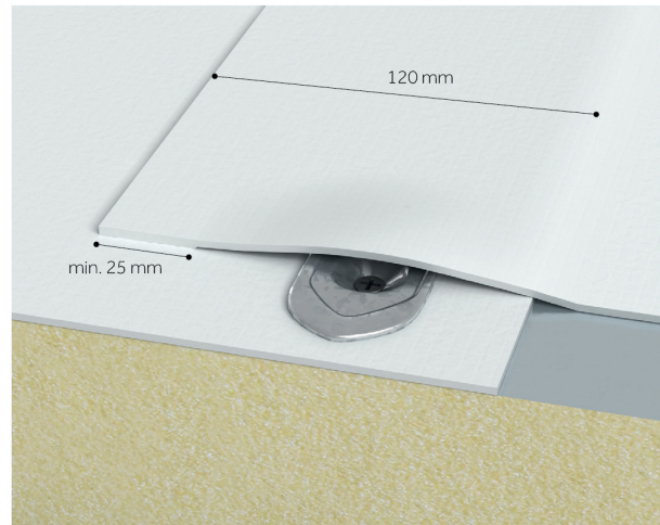
Side lap overlap with seam plate fixing.
