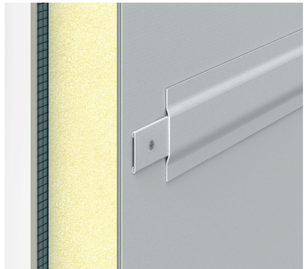
Figure 7. Intermediate fixing with strip of coated metal (shown) or fixation bar.
