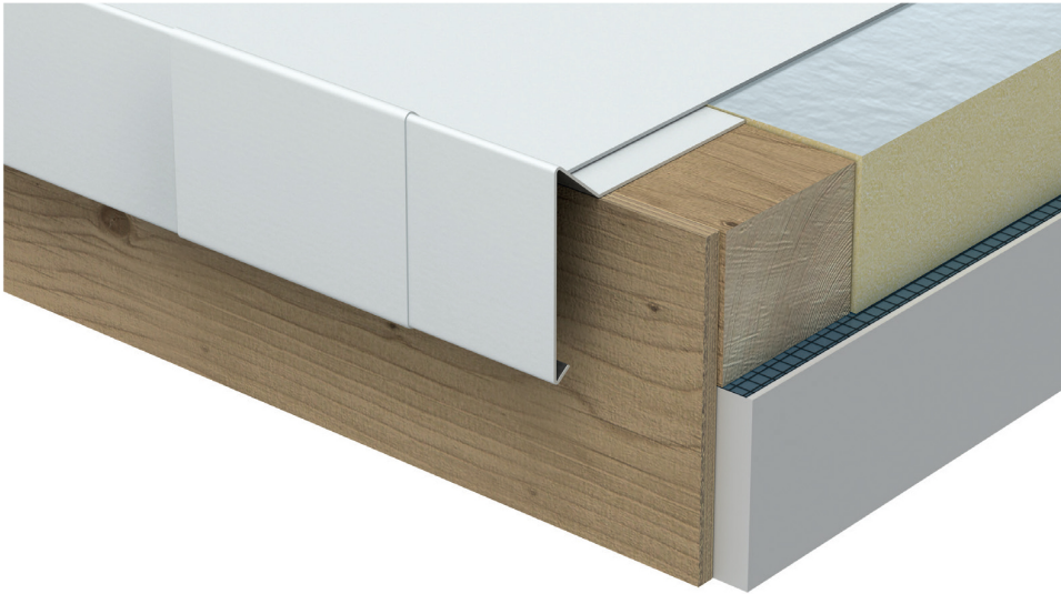
Figure 5. Drip edge detail with water check.
