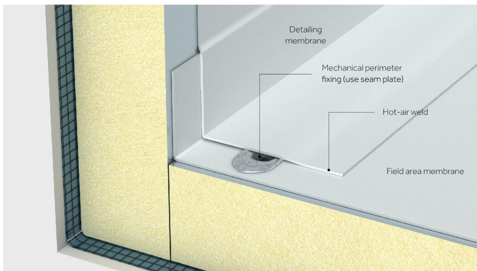
Figure 3. Perimeter fixing using fastener and washer.
