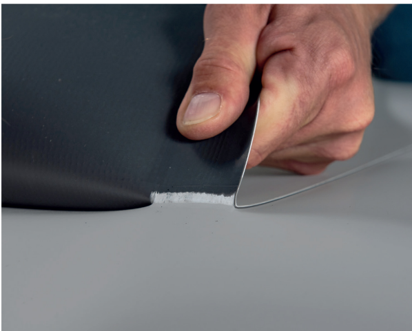
Figure 13. Carrying out a welding test.
