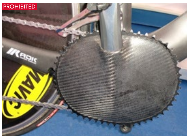
Photo. Example of a protective screen
