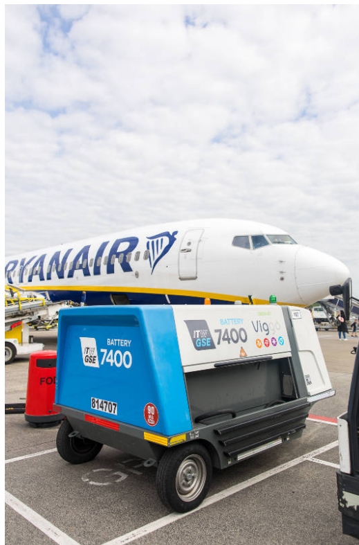
Elektrische Ground Power Unit
