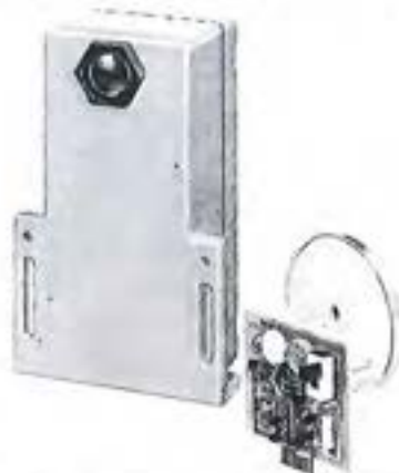
Self-contained : light source, photo receiver, amplifier, plug-in LOG logic card and output relay in a sturdy NEMA rated housing.
