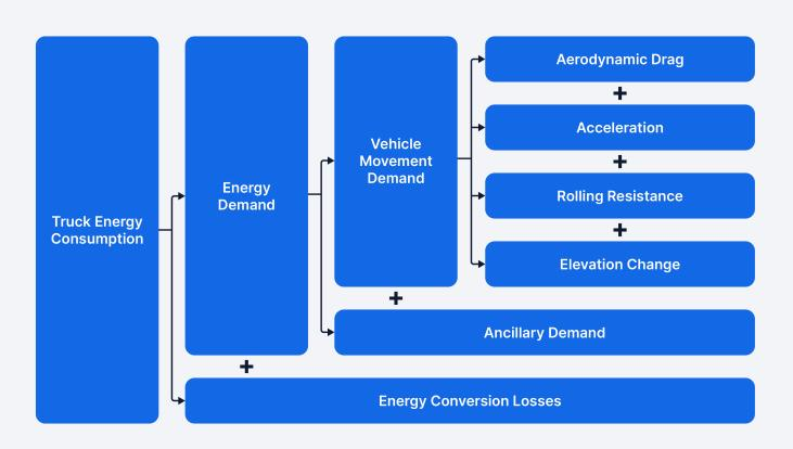
The majority of energy demand comes from moving the vehicle. The vehicle has to overcome **aerodynamic drag** as the vehicle pushes through the air, overcome **inertial force** any time the vehicle accelerates, overcome **rolling resistance** between the tires and road any time the vehicle is moving, and overcome gravity any time the vehicle is **increasing its elevation**. These different components can vary in relative impact depending on the context. For example:
