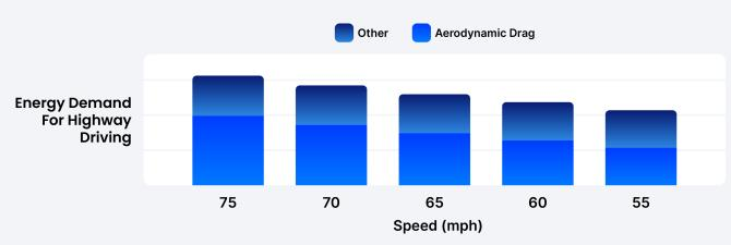
Figure 5: Highway driving energy demand vs. speed.
