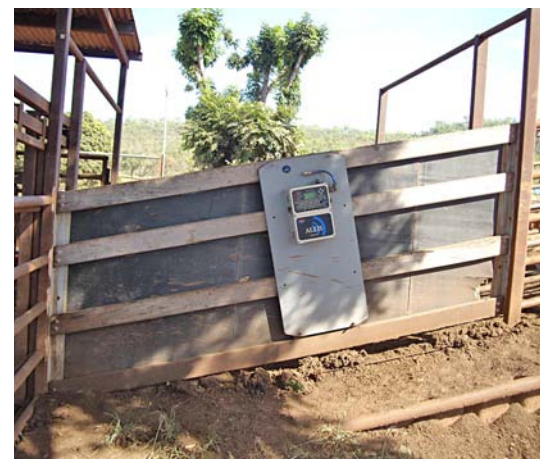
Automatic NLIS tag reader on loading ramp.
