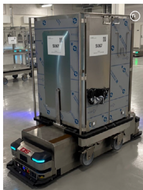
AGV (Automated Guided Vehicles) sjálfkeyrandi flutningsvagnar.
