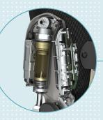
**C-Brace joint unit** With integrated Li-Ion battery and microprocessor
