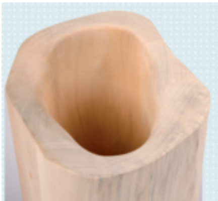
SF5P1=010 Smoothing the socket after copying
