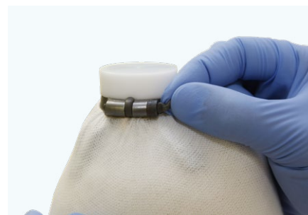
Isolate the corresponding areas of the objects that will be included in the laminate (e.g. screw heads, bare threads, joint surfaces) using the pre-formed Plastaband.
