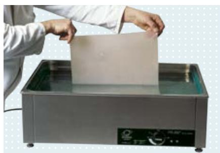
Place the pre-cut ThermoLyn Pedilon into warm water at approx. 60 °C in the 759P1=220 water pan. The material becomes transparent when it reaches its moulding temperature. Remove the pre-cut material with a wood spatula and allow the water to drip off.
