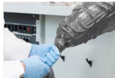
Use paper towels to clean the soaked 616F4 PVA bag on both sides and pull it over the model with the desired side (matte or gloss) facing outward. Tie off the PVA bag on the proximal end. Tie off temporarily in the distal region and create a vacuum. Mix the desired quantity of 617H119 Orthocryl lamination resin 80:20 PRO, without adding colour paste, with 2% hardener and fill into the PVA bag. Then tie off above the resin filling, without any air inclusions.
