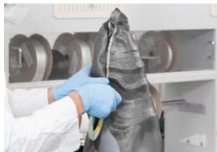
Attach one end of the layer of CarbonTEX PRO to the previously marked seam with 616F10=6 double-sided PVC adhesive tape and trim the excess material with the 719S21 carbon scissors. Then press any protruding fibres in place again. Repeat this procedure on the opposite side. To do so, apply a new strip of PVC adhesive tape to the cut edge of the CarbonTEX PRO side. Overlap and attach the second end of the layer of CarbonTEX PRO, trim the excess material and press any protruding fibres in place.
