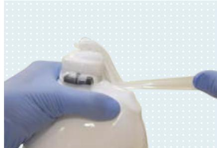
Apply 627B40 polyethylene adhesive tape around the areas that are to be opened after laminating; while doing so, excessive resin in these areas can be reduced with the pre-tensioned adhesive tape. With a given pre-tensioning, the adhesive tape can be twisted to a cord so that excess resin can also be reduced in areas that are difficult to access.
