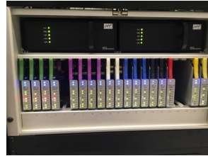
Pictured to the Left—"Under the hood" of the new 32KDS Central Audio Routing Switcher Below—back view cable harness
