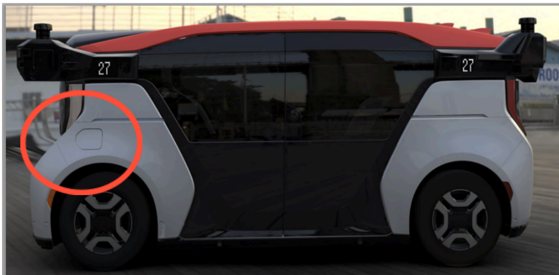
Location of charge port door on a Cruise Origin AV
