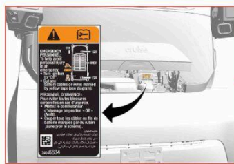
Battery warning label
