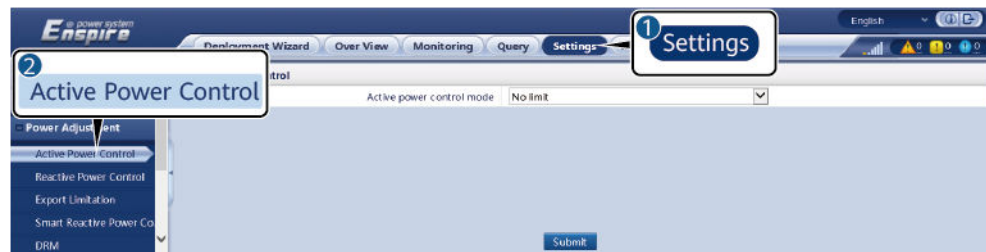
Figure 6-71 Active power control
