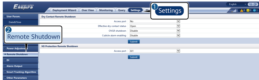
Figure 6-82 Dry contact remote shutdown
