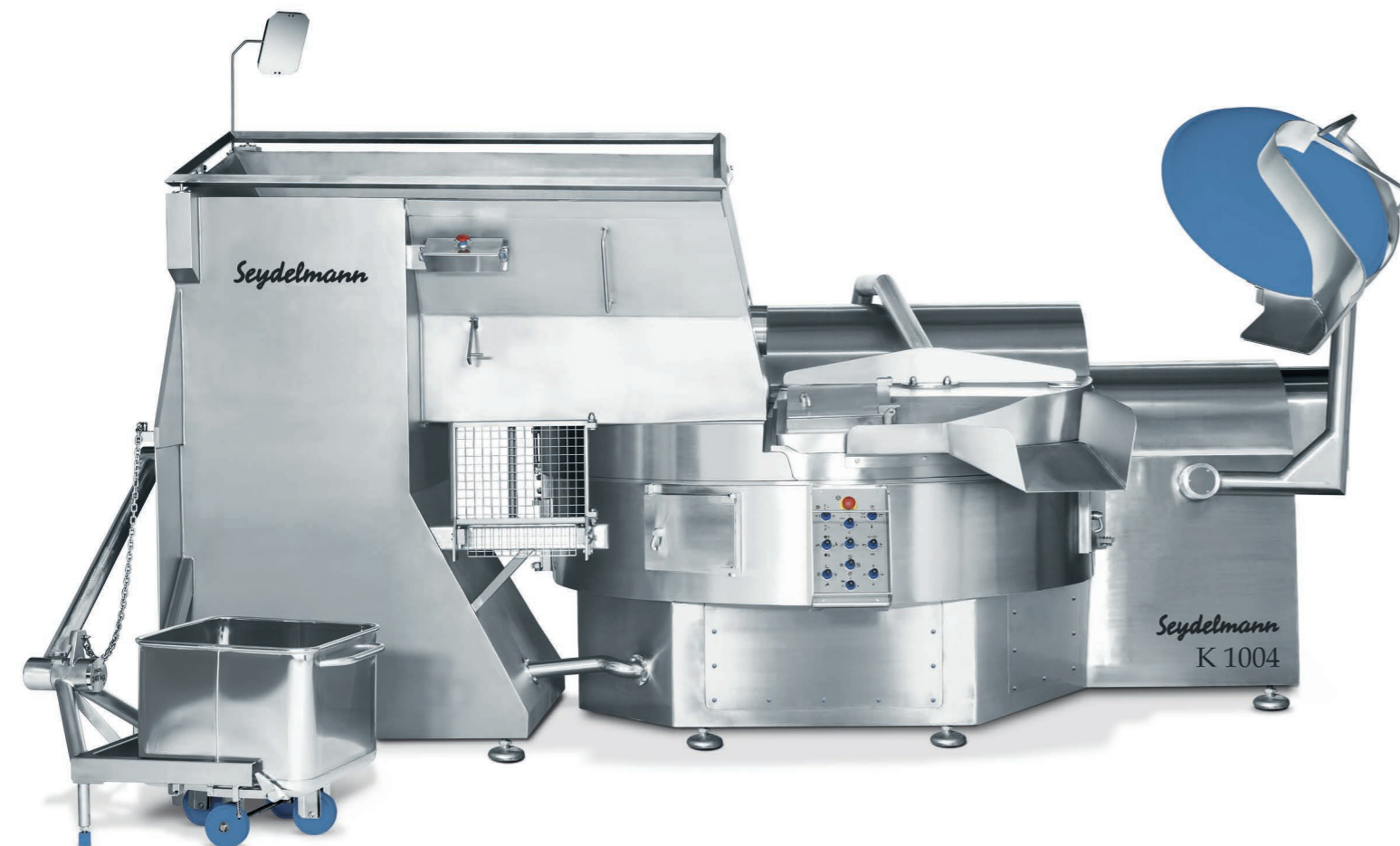
Loading of the K 1004 AC-8 via feeding storage with an integrated loading device for an increased time efficiency.
