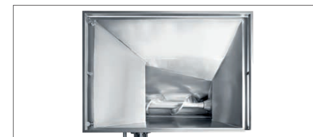
Feeding worm with breaking contour and cutting edge
