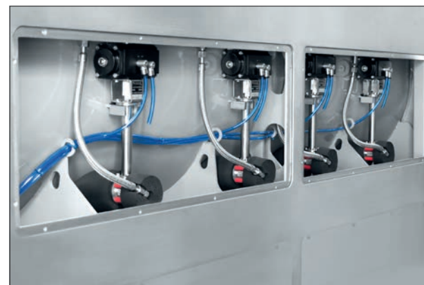
Cooling valves and nozzles behind the cover
