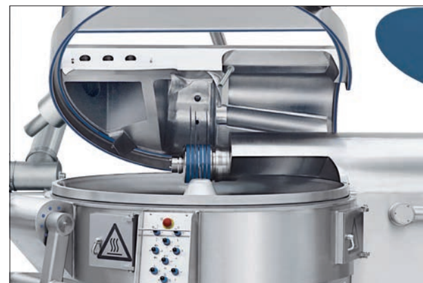
Cutter with cooling nozzles
