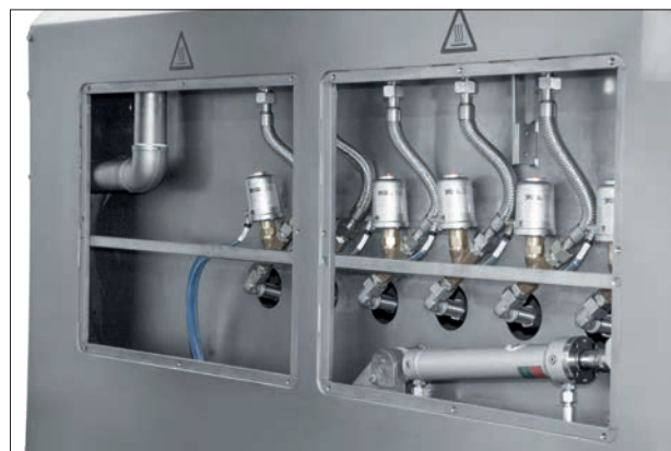
Integrated steam nozzle for direct heating
