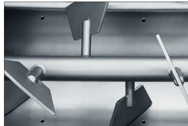
Mixer with mixing paddles and cooling nozzles
