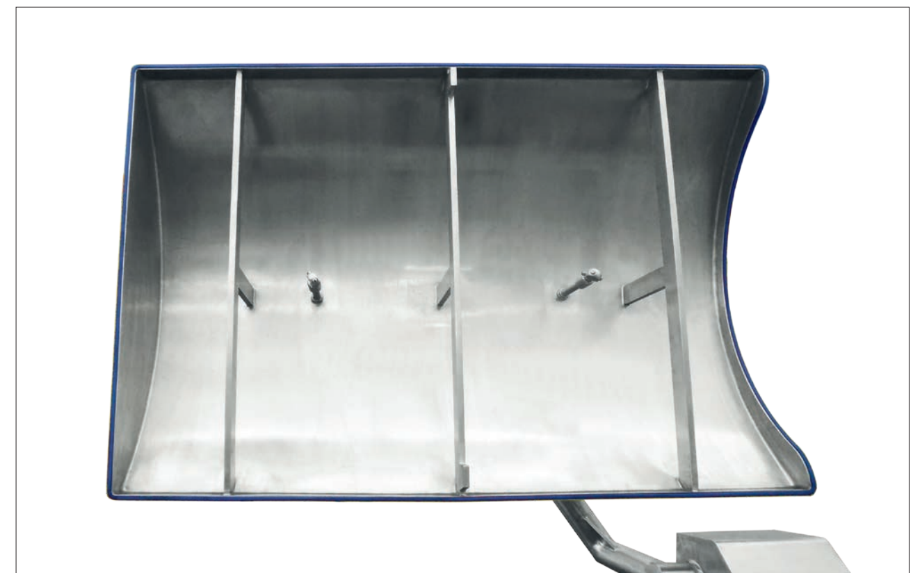
Cleaning nozzles integrated in the cover
