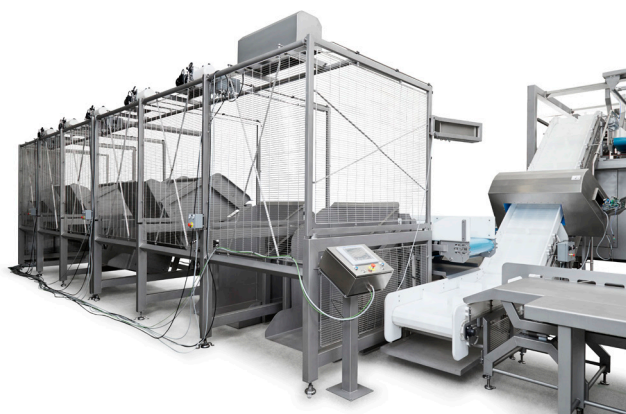
Weighing and batching station, seen from infeed side.
