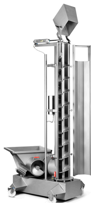
scansteel foodtech standard Giraff shown in cleaning position. Note the vertical screw is 100% accessible for cleaning (no hidden zones).
