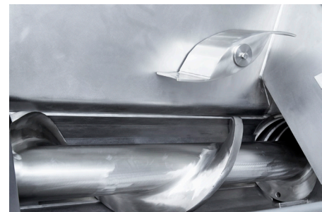
Cheese Feed Guide showed right mounted Electro polished feeding screw.
