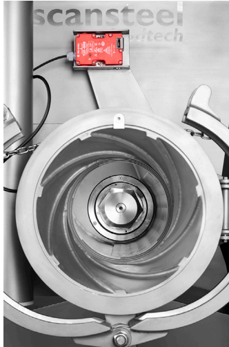
Cabinet without worm showing the flights of the lining.
