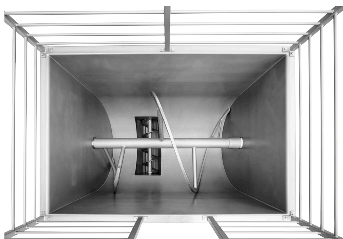
Top view of scansteel foodtech superGiraff, showing stirring/feeding device.
