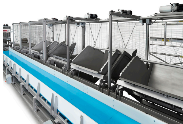
Weighing and batching station, seen from discharge side. Weighing belt positioned on load cells. Drip tray underneath to prevent dripping on floor.
