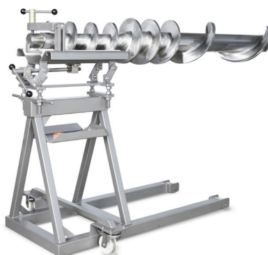
Removal of breaker worm for CombiGrind CG 225, CG 300, CG 300 Heavy Duty.
