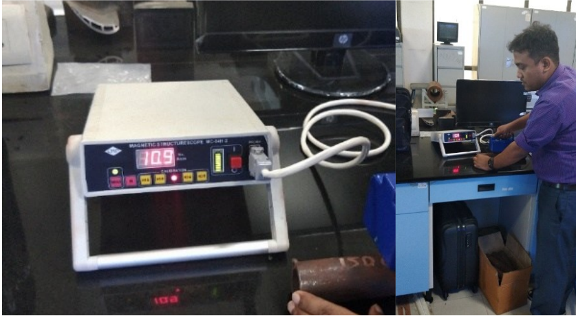
Fig 2. Photograph of MCF Measurement Test Setup Utilizing a Magnetic Structurescope.
