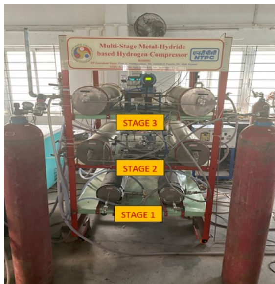
Fig. 11. Site photograph of the setup of the 3-stage MHHC.
