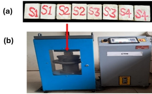
Fig. 2. Cube Cast from S1 to S4 before and after CO 2 sequestration (a) and Enkay 2000N compression testing machine (a).
