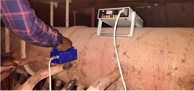
Fig 9. In-Situ Evaluation of PWHT Effectiveness for T91 Boiler Tubes Through MCF Measurement.
