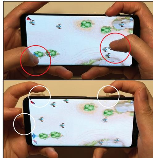
Fig. 13. **Mobile gaming.** (top) When controlling a game on a mobile device, the player’s fingers often occlude the display (e.g., in red circles) and cause disruption. (down) Vidgets interface (in white circles) enables the player to control game more efficiently without occluding the screen.
