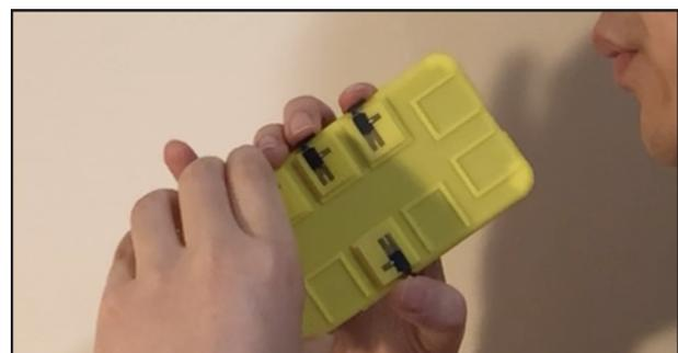
Fig. 14. **Saxophone app.** We demonstrate a 4-key “smartphone’s saxophone”. Each Vidgets button serves as a saxophone key. By detecting the downstroke and upstroke of each Vidgets button, this smartphone application can recognize which keys (and key combinations) are pressed and play the corresponding music notes.
