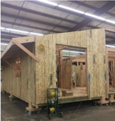
In the factory, the roof is constructed with overhang and then flipped onto main roof for shipping.
